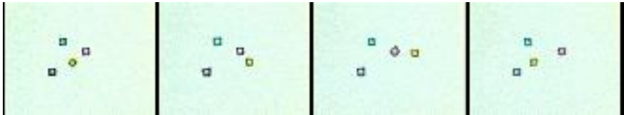
Fig. 10. The third robot is exploring without success its row and when it goes out of the board, it goes up signalling the second robot. This one finds a new free patch while the third robot is going back to the start position
